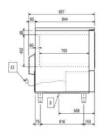
Drain Electrical inlet (power)
